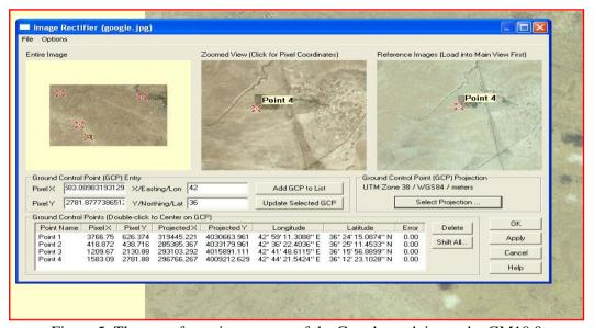
Figure 5: The georeferencing process of the Google earth image by GM10.0
