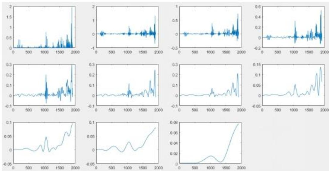
Figure5: From left to right, from top to bottom is respectively the original signal, IMF2\_c, IMF3\_c, ..., IMF10\_c, IMF11\_C of JV.
