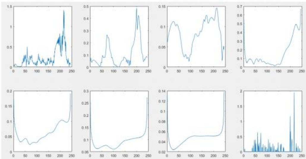
Figure9: Time - amplitude figure of each IMF of JV after Hilbert transform
