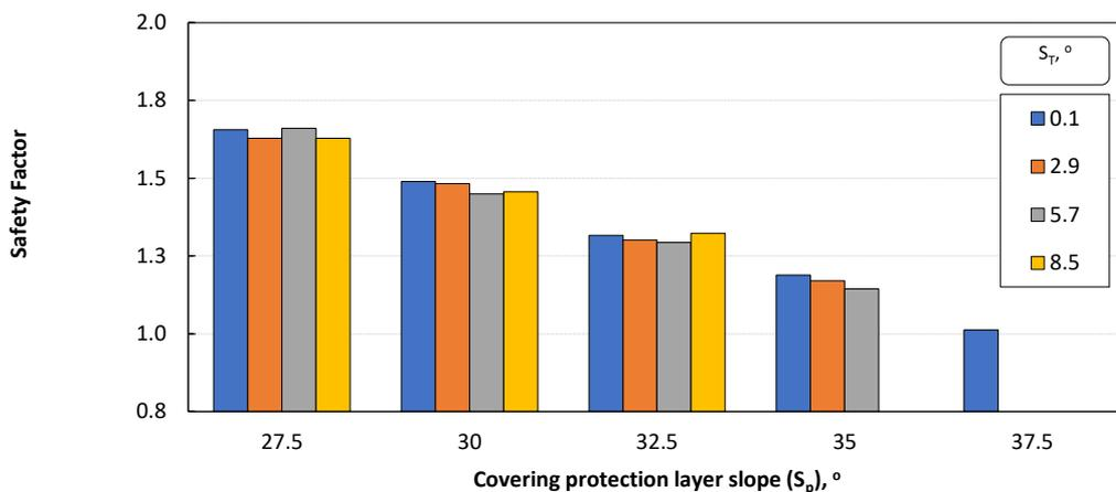
**Figure 4: Safety factors derived from slope stability analysis for different angles of the slope of the top liner system ( $S_T$ ) and of the slope of covering erosion-protective layer ( $S_p$ ), [10].**
