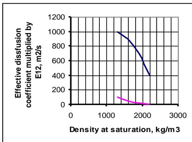
**Figure 19: Measured effective diffusivities of smectite clay. The upper curve refers to monovalent cations and the lower to anions.**
