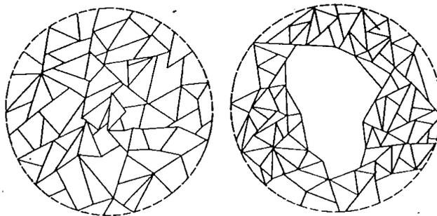
**Figure 17: Coagulation of clay particles. Left: Structurally homogeneous clay network. Right: Coagulation by increased electrolyte concentration in the porewater.**
