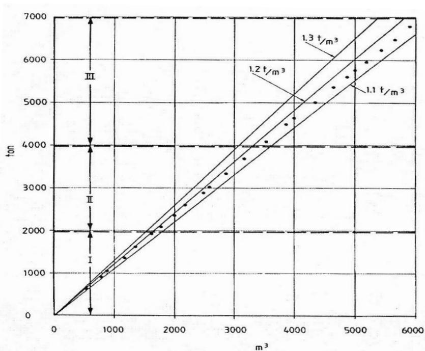
**Figure 11: Bulk density of the granulated clay fill determined in the course of the placement made by use of a hopper located about 50 m over filled mass (left). The density is expressed in tons per cubic meter in the graph [19,20].**
