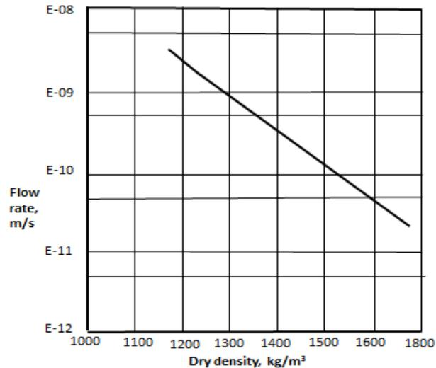
**Figure 7: Approximate average percolation rate of water passing through a 0.5 m thick clay liner of clay with 20 % montmorillonite content as a function of the dry density. The assumed hydraulic gradient is 10 m/m.**
