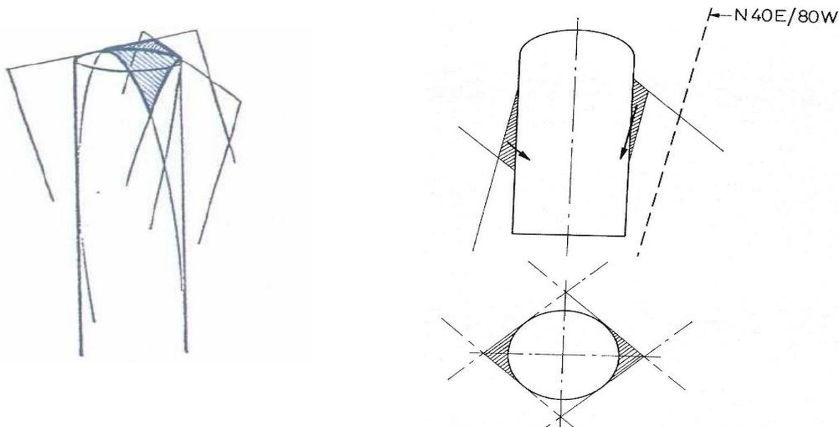
**Figure 15: Unstable rock wedges formed by crossings of steeply oriented fracture zones or discrete fractures. The right picture refers to the room hosting the big silo in Figure 10. The crossings are major hydraulic conductors.**
