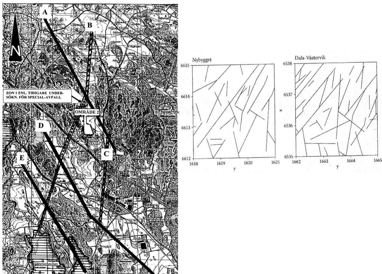
**Figure 13: Fracture zones in granite identified by geologic and topographic site selection analyses. a) Common pattern of fracture zones (edge length 0.7x1.1 km). b) large-scale patterns of major fracture zones in granite (left) and in gneiss (Scale in kilometers).**
