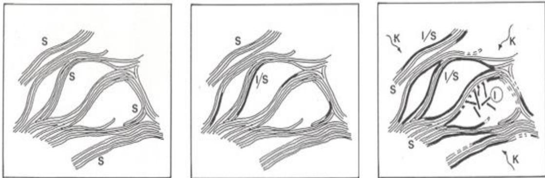
**Figure 21: Smectite-to-illite conversion via mixed-layer I/S formation and/or direct precipitation of illite. Dark contours represent precipitations of silica and/or illite. S is smectite, I is Illite, and K is potassium [21].**
