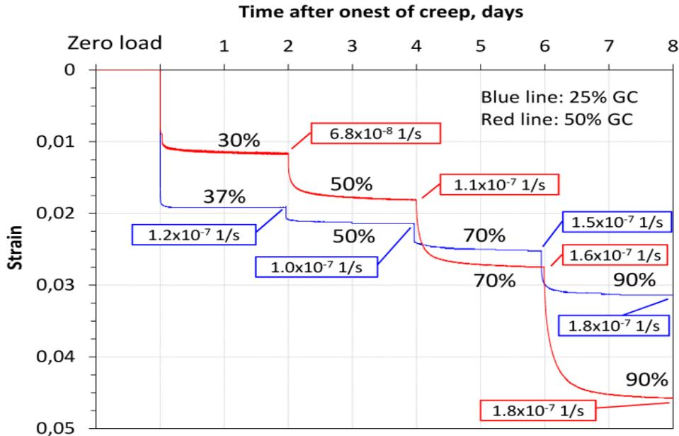
**Figure 5: Creep behaviour of mixtures with 25 and 50% “Green clay” for step-wise loading (ratios indicate load increments in percentage of the unconfined compressive strength). The numbers in frames indicate, in potential form, the strain rates at the end of each loading step [10]. The stabilizing effect of extra sand, represented by the blue curves in the diagram, is obvious.**
