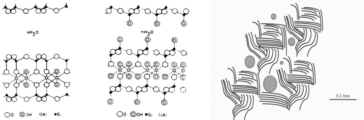
**Figure 16: The smectite mineral montmorillonite. Left: Crystal structure models with interlamellar water. Right: Schematic microstructural model of hydrated clay with bulk density  $1,800\text{-}2,000\text{kg/m}^3$  at water saturation. For the lower density the bar is  $0.1\text{ mm}$  and for the higher it is  $0.01\text{mm}$ . Circles are channels with water and dilute clay gels [11].**
