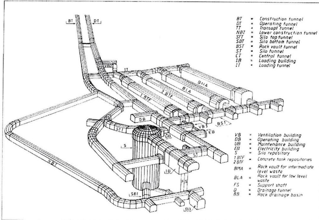
**Figure 9: Overview of SKB's facility for disposal of LLW in tunnels and of LLW and ILW in a concrete silo built in a big cavern (After SKB).**
