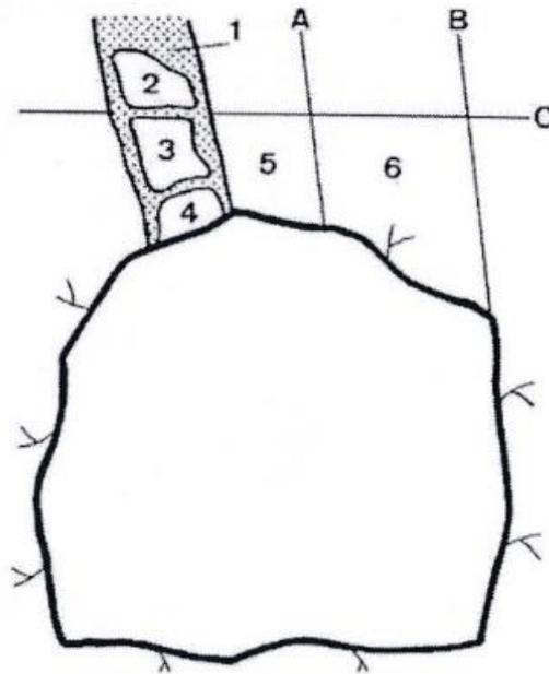
**Figure 14: Tunnel section with seams of clay-weathered crystalline rock and potentially unstable rock blocks (1-4). A-C are fractures with insignificant or no gouge but with a potential to weaken by weathering.**
