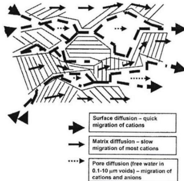
**Figure 18: Smectite clay microstructure with dense particle aggregates shown as hatched areas. Surface diffusion takes place along the exposed free surface of aggregates of stacks of smectite lamellae. Matrix diffusion occurs within the aggregates, primarily by cation diffusion in the interlamellar space, while pore diffusion takes place in wider voids.**
