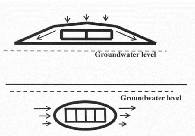
**Figure 1: Two options for LLW and ILW disposal with clay liners. Upper: on-ground disposal (“near surface option”). Lower: underground disposal (“geologic option”), both requiring clay isolation of concrete vaults containing waste. Arrows indicate water flow.**
