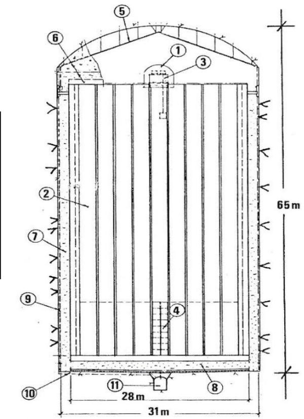
**Figure 10: The disposal facility at Forsmark, Sweden showing the big silo for disposal of LLW and ILW and the system of tunnels for storage of very low-active radioactive waste (After SKB).**
