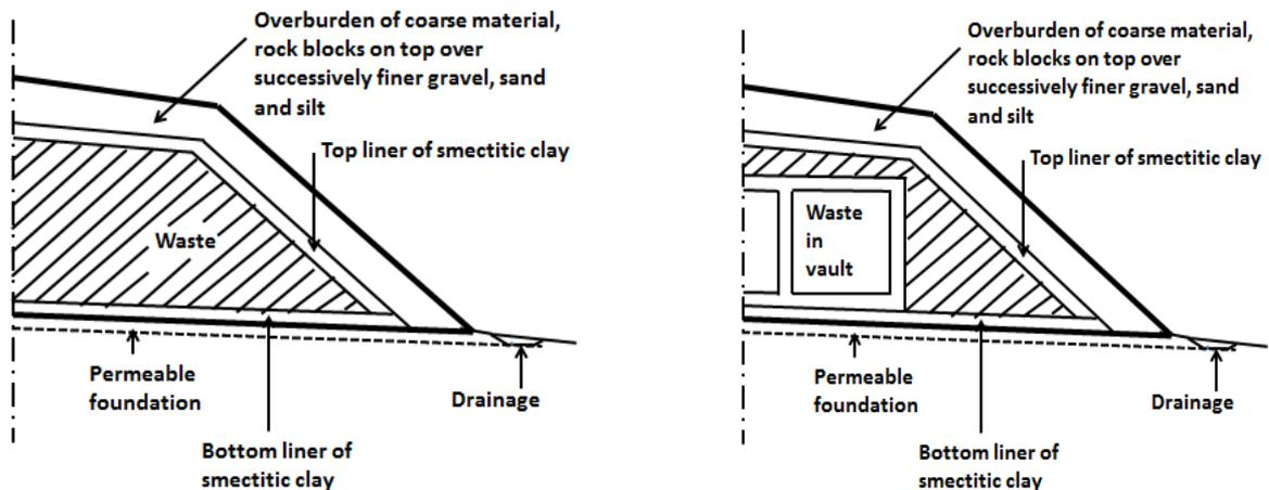
**Figure 2: Schematic sections of on-ground repositories for LLW and ILW. Left: Simple landfill for very low-level waste. Right: Ordinary LLW and ILW placed in concrete vaults [1].**
