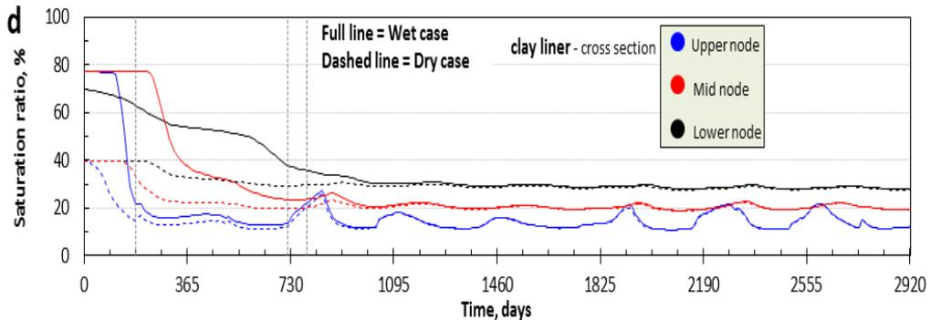
**Figure 6: VADOSE/W simulations for wet and dry conditions of the top liner in arid desert illustrate the expected variation in saturation ratio in the upper part of the top liner (“d”), [10].**
