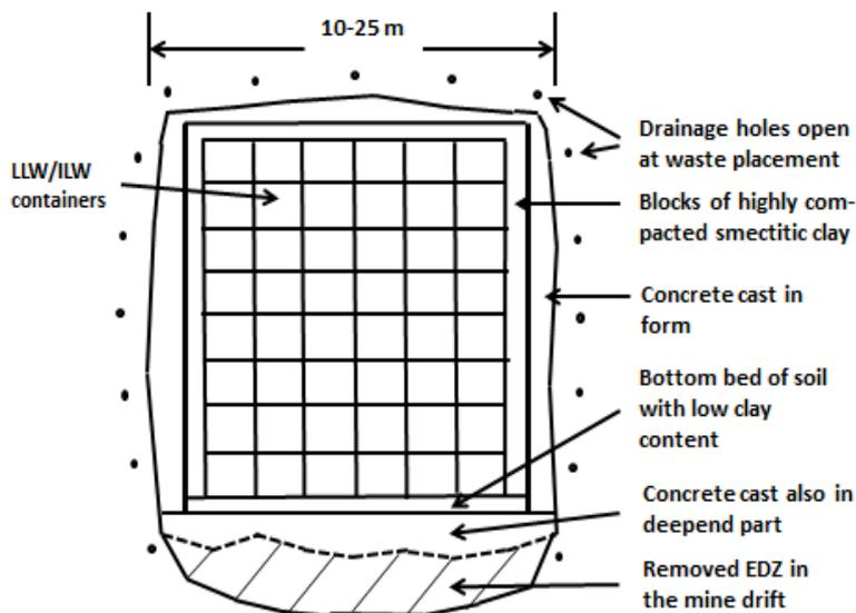
**Figure 8: Principle of effective isolation of LLW/ILW in large blast-excavated rooms or in abandoned mines. EDZ is permeable fractured rock formed by blasting [11].**
