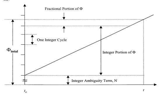
Therefore, the total phase range can be written as the sum of the measured phase observation and the integer ambiguity term, N(t). The measured phase range for the carrier phase observable is shown by the following equation:
