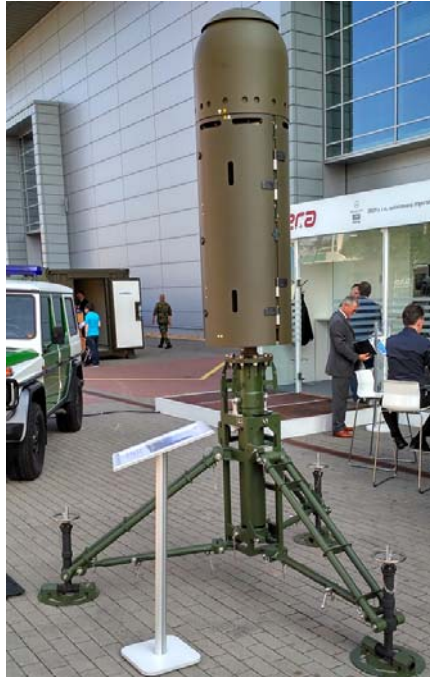
Figure 3: The passive ESM tracker VERA NG of the Czech ERA at IDET2017, Brno, Czech Republic. This is an example of an Emitter Locating System, which exploits emissions of the target to locate it. If a target is under complete emission control, it will not be detected by such a system.
