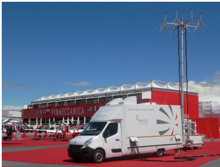
Figure 2: The AULOS Passive Radar of Leonardo (ex SELEX SI, the Finmeccanica group) [17]
