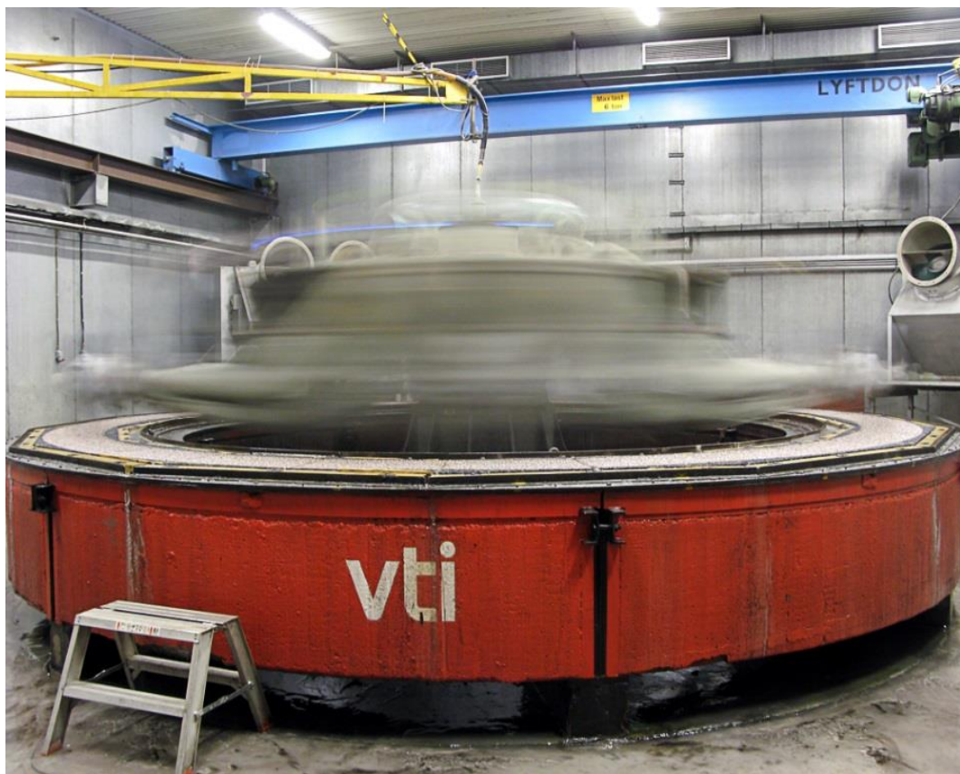
Figure 1: The VTI road simulator. Photo: Mats Gustafsson, VTI.
