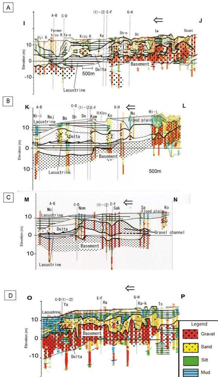
171 Figure 5: Geological cross-sections (N-S direction) of the lower reaches of the Kizu River, showing lithology
