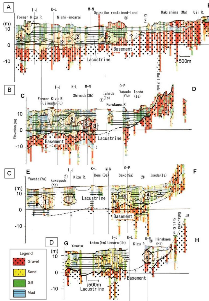
161 Figure 4: (A)–(D) Geological cross-sections (W–E direction) of the lower reaches of the Kizu River, showing
