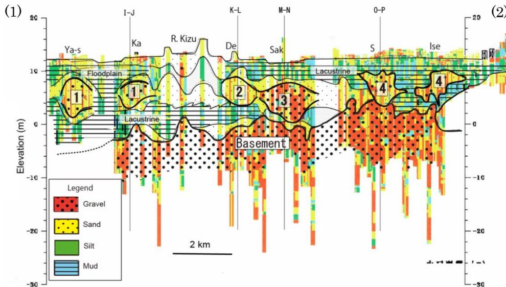
140 Figure 3: Geological cross-sections (W-E direction) of the lower reaches of the Kizu River, showing lithology
