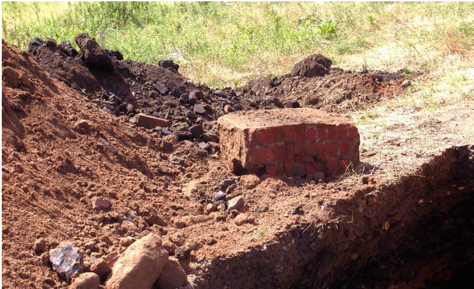
Fig. 3 Shallow excavation showing fills comprising discarded construction materials.
