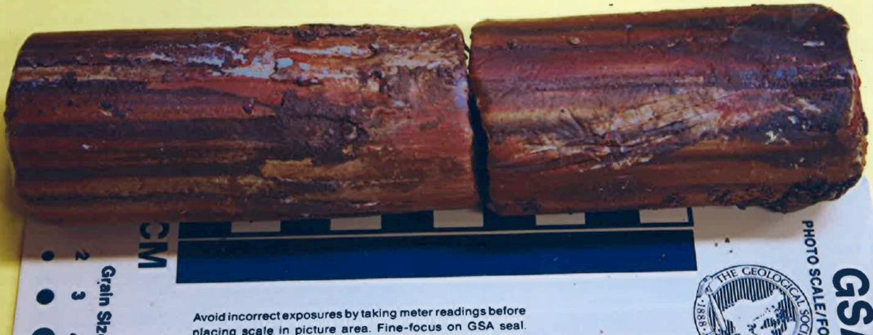
Fig. 8 Major lithologic unit above the solid bedrock is dominantly composed of variegated, moderately to highly compact silty clay; often recording higher N or SPT counts.
