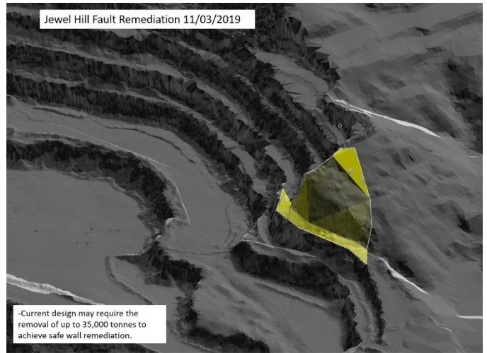
Fig. 1. Plan to excavate out remaining unstable ground
