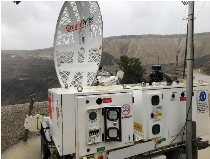
Fig. 1. Groundprobe SSR used to monitor pit high walls
