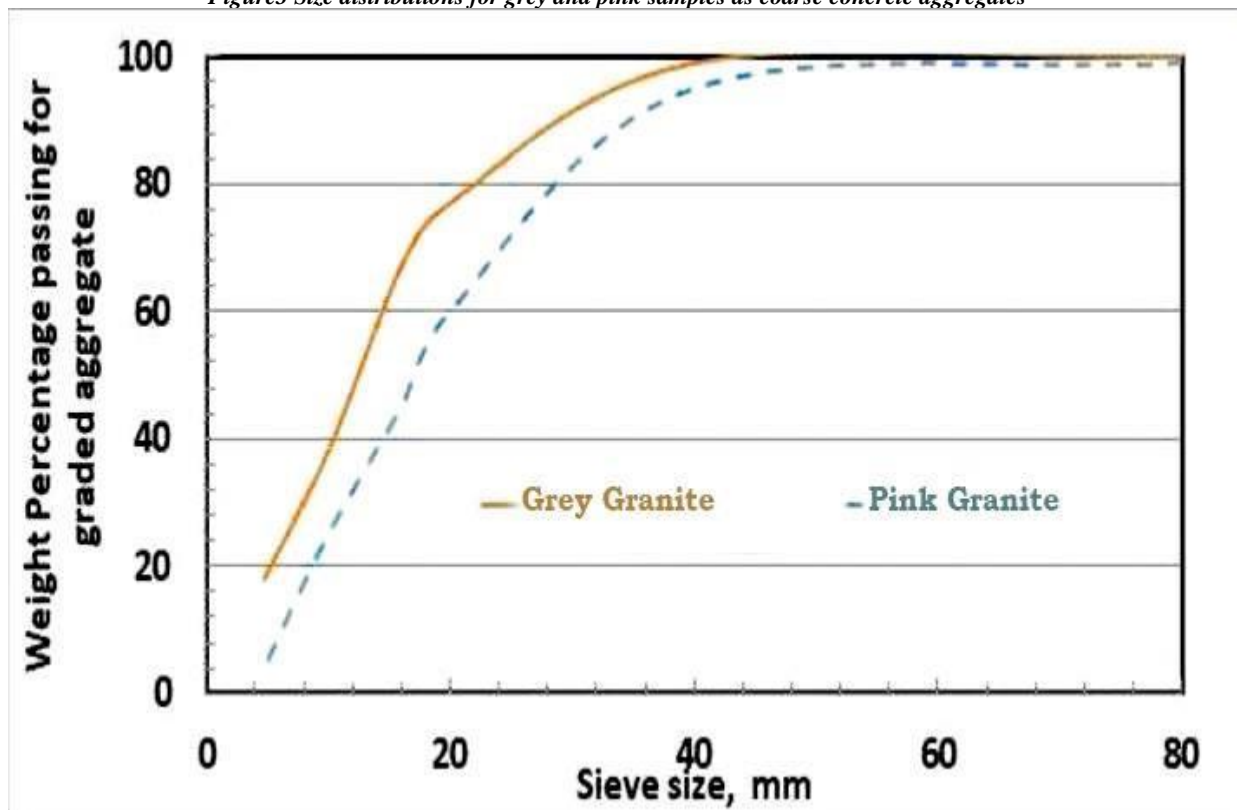
Figure3 Size distributions for grey and pink samples as coarse concrete aggregates
