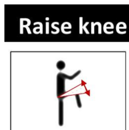
Figure 6: Specific margin (in red) for thigh elevation when raising the knee. The hip angle for the H posture should vary within this margin ( 120^\circ \pm 8,3^\circ ) [19] for the objective set to be validated.
