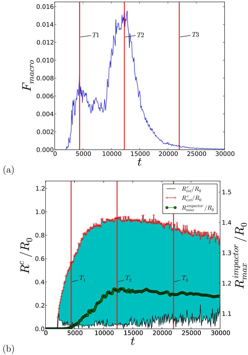
Figure 6: a) Time history of the load  $F_{macro}$ , imposed onto the target by the impactor; b) time history of the contact radius  $R_{int}^c$  and  $R_{ext}^c$ , between the target and the impactor, as well as the time history of the maximum radius of the impactor  $R_{max}^{impactor}$ .
