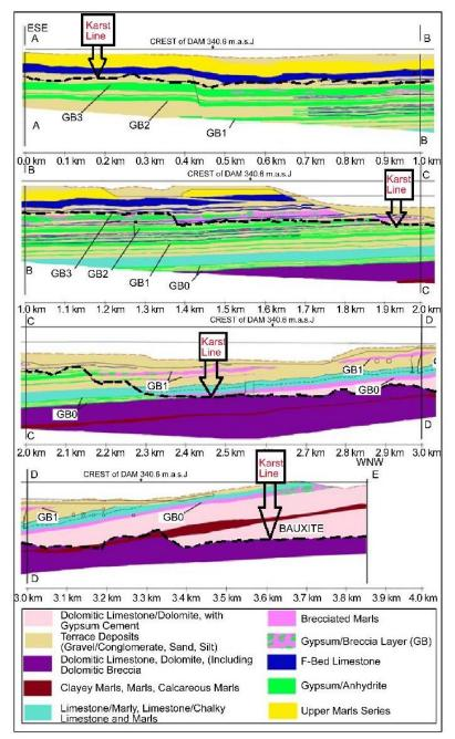
Figure 8: Assumed Karsts line in Mosul Dam foundations (From [1])
