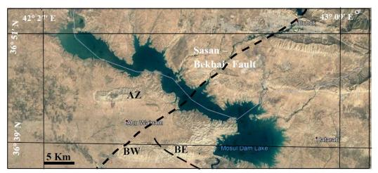
Figure 4: Google Earth image of Mosul Dam and Lake. Note the deep seated Sasan – Bekhair Fault. Anticlines: BE = Butma East, BW = Butma West, AZ = Ain Zala,
