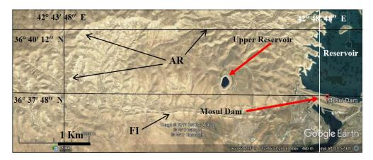
Figure 2: Google Earth image of Mosul Dam site. Note the anticlinal ridges (AR) and the Flat irons (FI)
