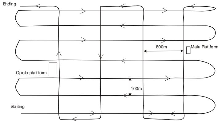
Fig. 6: Traverse pattern during marine surveys
