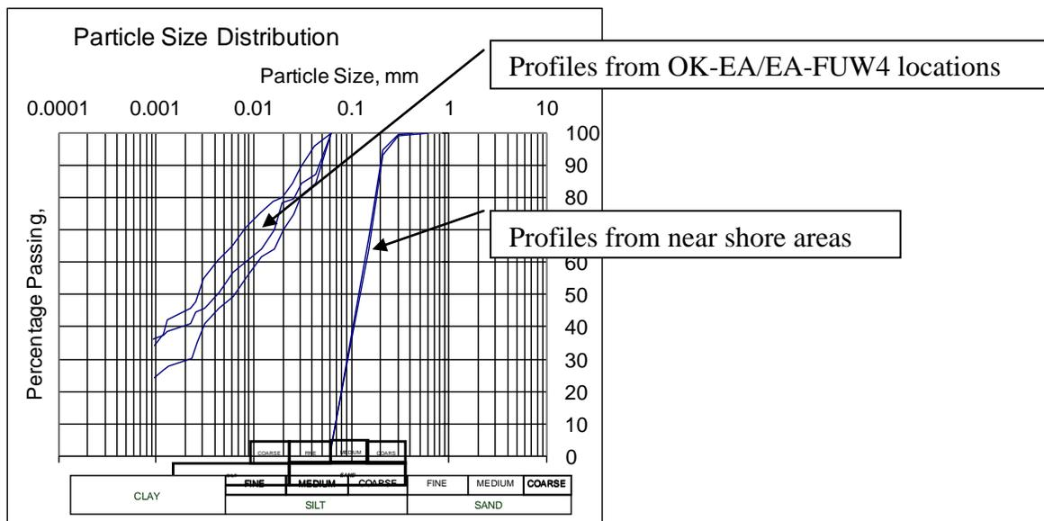
Fig. (9) Particle size distribution for shore area and deeper OK-EAS and EA-FUW4 locations
