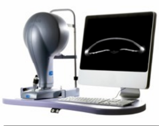
Figure 1: Sirius Scheimpflug camera
