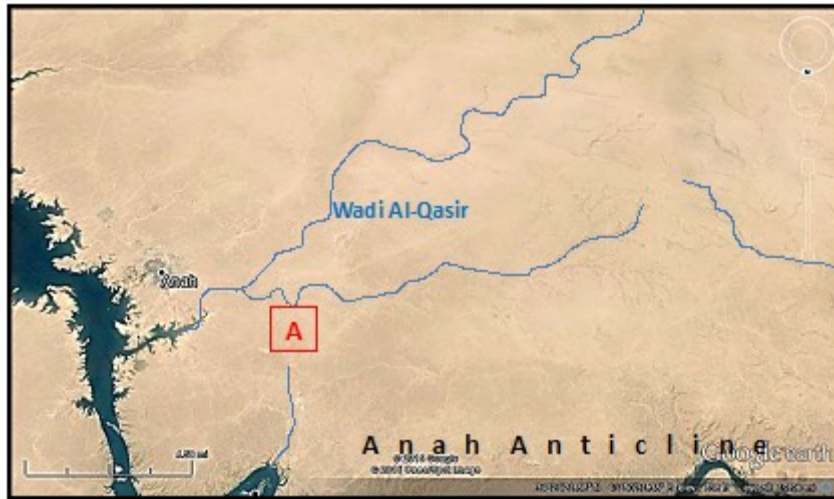
Figure 13: Google Earth image (Facing south) showing wadi Al-Qasir with drainage parallel to Anah anticline. Possibly the lower branch of wadi Al-Qasir was crossing Anah anticline at point A , the remaining course is still there; leading to the river.
