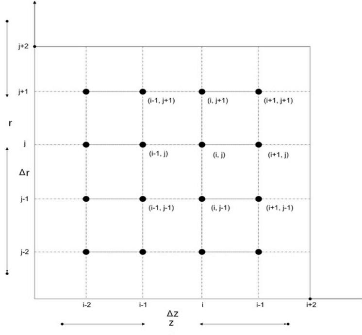
Figure 3: Finite Difference Grid for hollow cylinder
