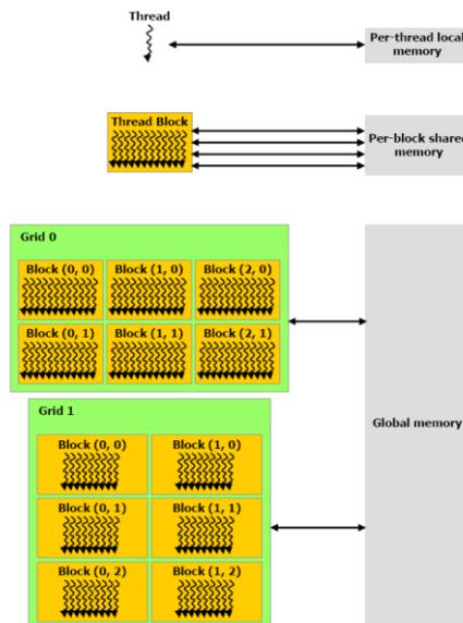
Figure 1: GPU Memory Architecture [2]
