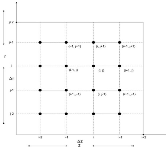
Figure 2: Finite Difference Grid for solid cylinder
