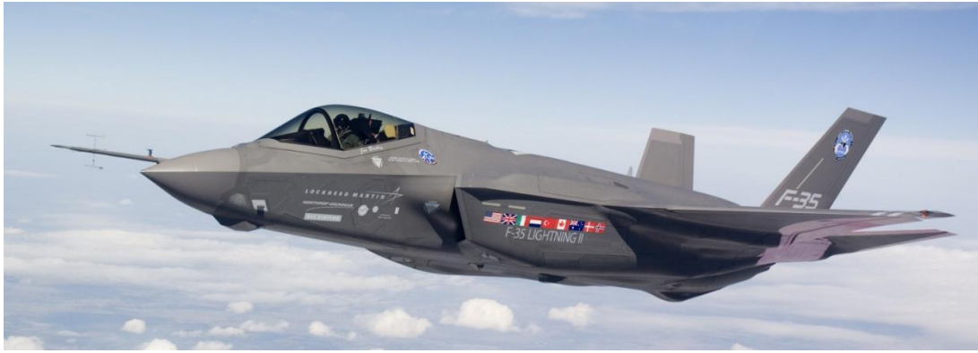
Figure 3. The F-35A Lightning II during development phase. A single-engine, 5 th gen. multirole fighter with stealth capabilities, set out to repeat the success of the F-16 ([4]).
