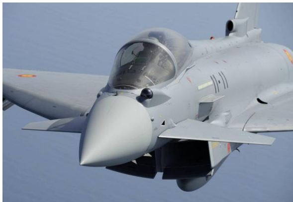
Figure 11. The PIRATE IRST system on a Spanish Air Force Eurofighter Typhoon.
