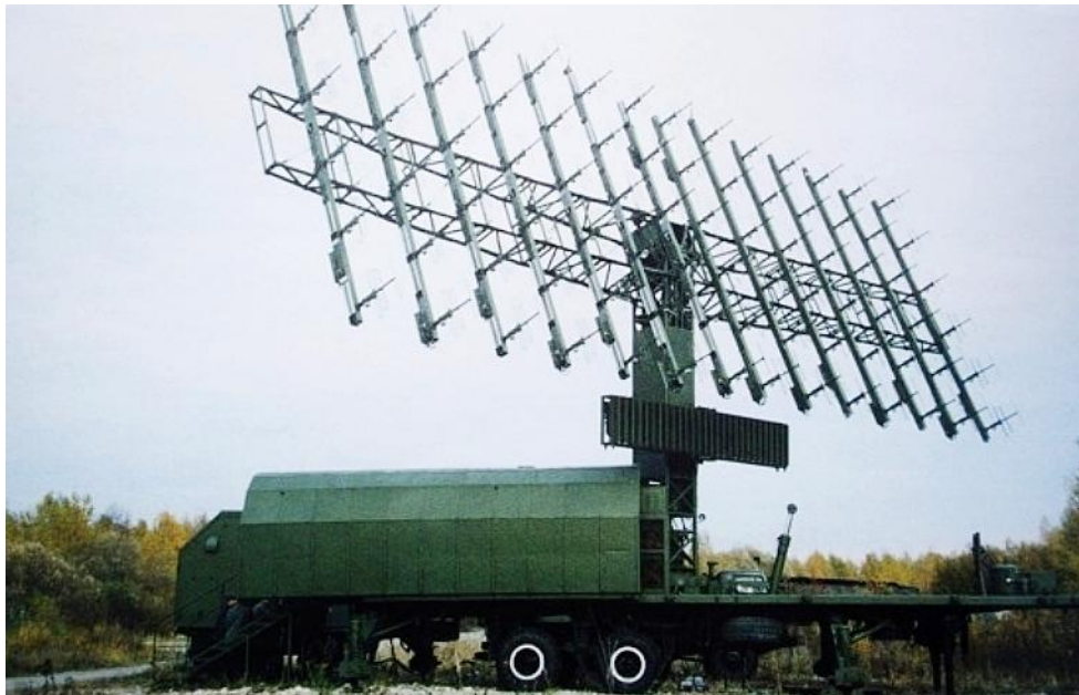
Figure 9. The 3D VHF AESA Radar 1L119 NEBO SVU, developed by NNIIRT (Russia) and offered for export by Rosoboronexport (the sole state export entity for defence products in Russia). It is a mobile, long range surveillance radar, featuring modern technology, able to detect stealth aircraft from considerable distances ([80]).
