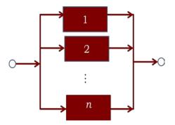
Figure 3: A parallel system of n component information operations
