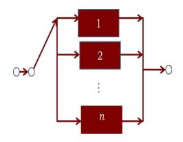
Figure 4: A parallel system of *n* component information operations with standby redundancy
