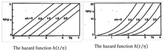
for Weibull distribution with  $\beta = 2.0$  for Weibull distribution with  $\beta = 3.0$ Figure 10: Information operations hazard functions  $h(t/\eta)$  for Weibull distributions
