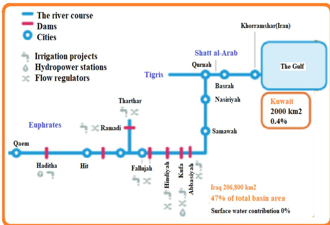
Figure 17: Iraqi exploitation of the Euphrates water system. (Source: [12]).
