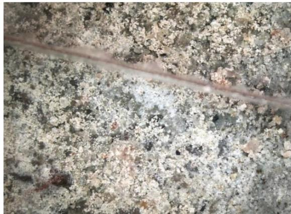
**Figure 25: Microstructural constitution of montmorillonite-rich clay (MX-80) sample saturated with 10% CaCl<sub>2</sub> solution and hydrothermally treated at 95°C, placed in a shear box for shearing along the joint between the two box parts (brown line). Magnification 200x. On-falling LED light.**
