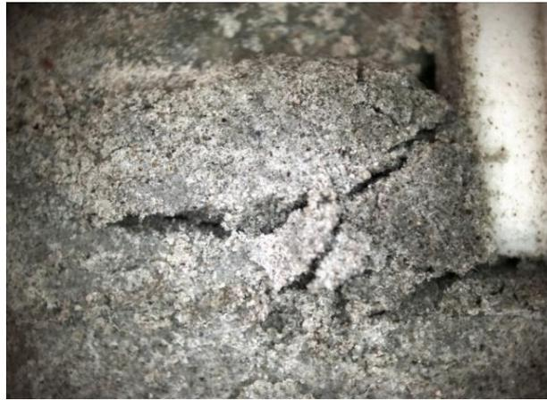
**Figure 26: The clay sample in Figure 25 sheared after hydrothermal treatment at 95°C. The white object to the right is one of the shear box halves. The fracturing that took place in conjunction with dilatancy at about 20 % strain in the sheared direction (right to left) demonstrates brittle behaviour and lack of self-sealing ability of the clay. Magnification 200x. On-falling LED light.**
