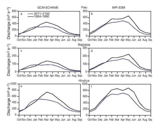
Figure 7: Mean monthly discharge (m3/ s) simulated by the HD model for (a, b) Palu,(C,d) Baağişas, and (e, f) Hindiya for the reference (black solid line) and future (blue dashed line) periods. Forcing- (a, c, e) GCM-ECHAM5; (b, d, f) MPI-ESM. (Base period 1969-1990, Future period 2071-2100)
