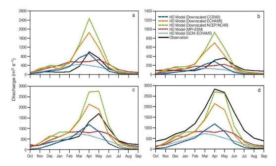
Figure 6: Mean monthly discharge for (a) Palu, (b) Baağiştas, , (c) Hindiya and (d) Baghdad stream flow gauging station (black continuous line) and the HD model simulation results (dashed lines) forced by GCM-ECHAM5 (blue), MPI-ESM (red RCM-NCEP/NCAR (orange), RCM-ECHAM5 (green) and RCM-CCSM3 (dark blue). Note differences in y-axis scales (1961-1990).
