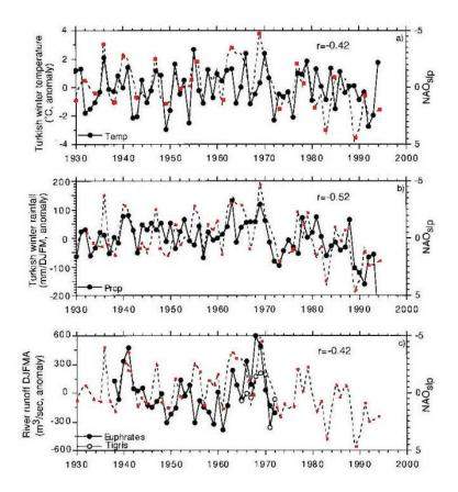
Figure 5: Correlation between the NAO<sub>SLP</sub> index, (a) Turkish winter temperature index, (b) Turkish winter precipitation index and (c) DJFMA average stream flow of the Euphrates (filled circles) and the Tigris Rivers (open circles) (note: the NAOSLP index has been multiplied by \_1.
