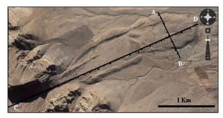
Figure 3: Flash Earth image, facing south showing the Qara Chattan Landslide.  $(A-B \text{ is a cross section to show the curvature of the slid mass,} \\ \text{and } C-D \text{ is longitudinal cross section}$
