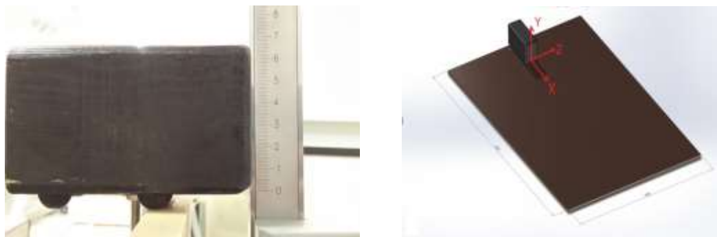
Figure 1: Car model used during the experiments (Left) and the Cartesian coordinate system with incoming flow from top left to bottom right (Right)
