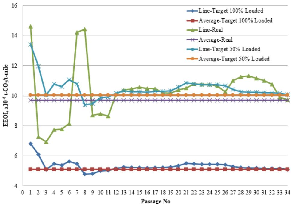
Figure 2: EEOI calculations for different loading of M/V Ince Anadolu.
