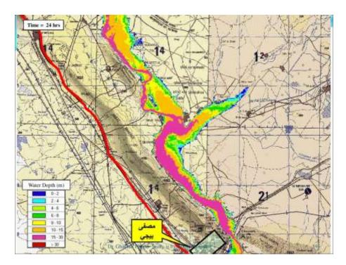
Figure 9: Wave at Makhul (Just North of Baije) after 24 hours of Dam Break
