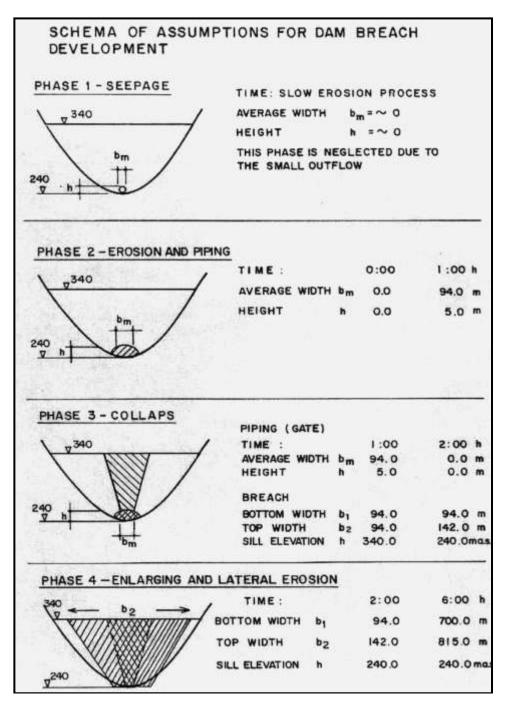
Fig 2: Stages of breach development
