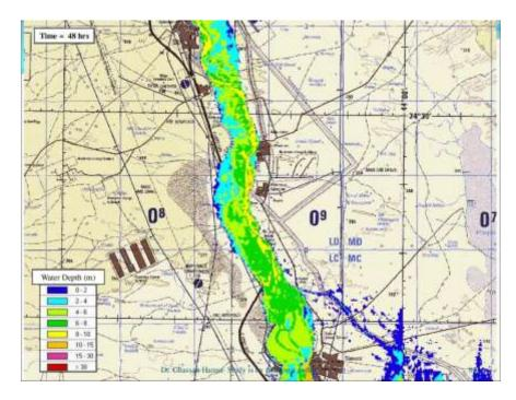
Figure 14: Wave at Sammara after 48 hours of Dam Break.
