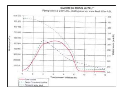
Fig. 3: Dam breaks Hydrographs obtained by FLORIS and DAMBRK UK software [9].
