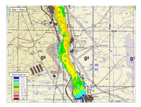
Figure 13: Wave at Sammara after 29 hours of Dam Break
