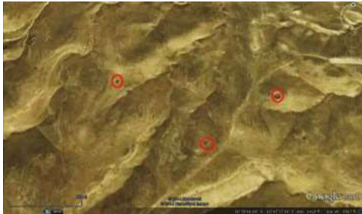
Figure 8: Enlarged Google Earth image showing many sinkholes (Dark spots encircled by red color) in the upstream area of the dam site [3] [4] [5] [6]
