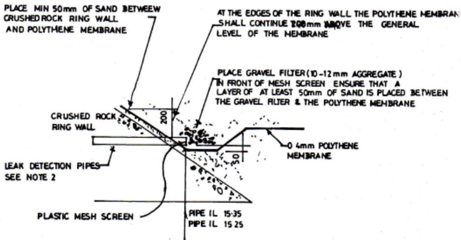
Figure 9: Details of Polythene membrane gravel filter and leak detection pipe connection
