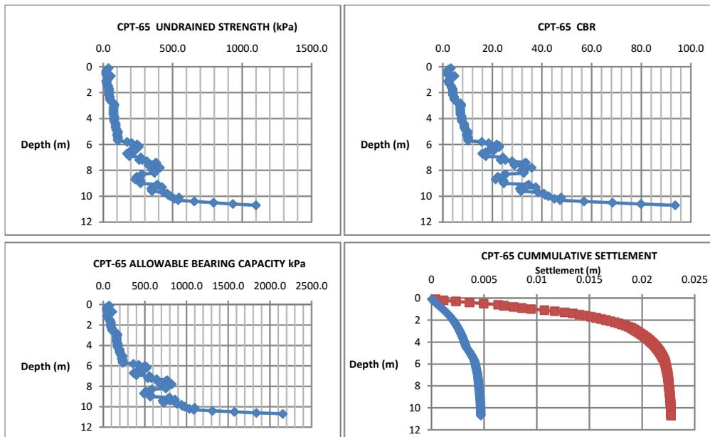
Figure 5: Vertical profiles of undrained strength, allowable bearing pressure, California Bearing Ratio (CBR) and cumulative settlement distribution at location CPT65
