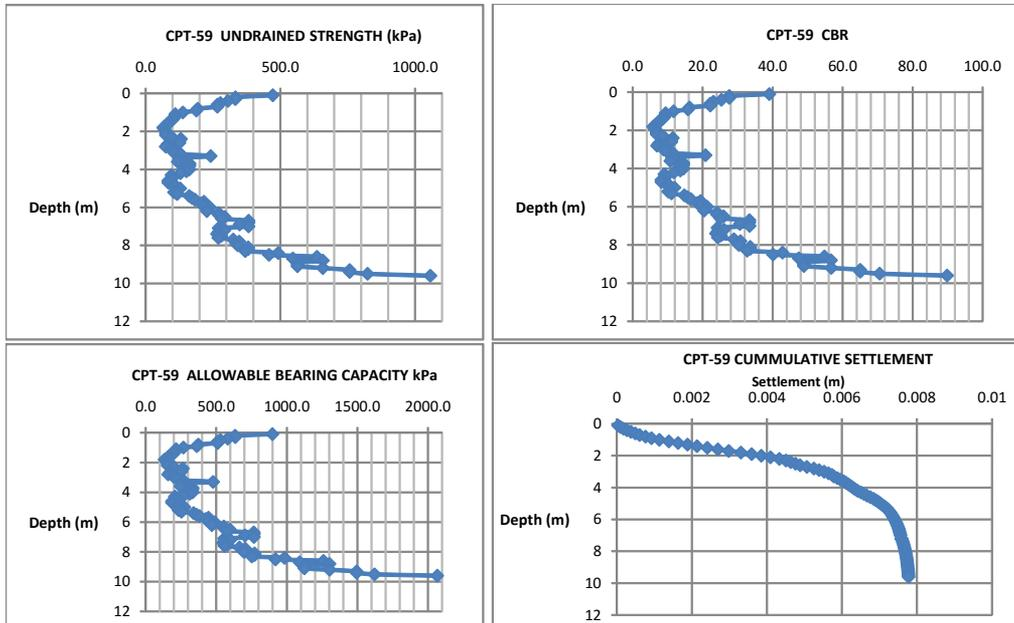
Figure 4: vertical profiles of undrained strength, allowable bearing pressure, California Bearing Ratio (CBR) and cumulative settlement distribution at location CPT59
