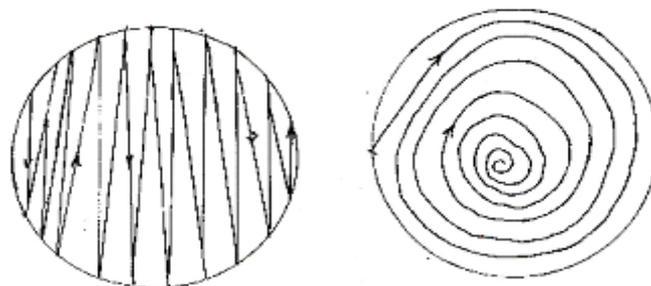
Figure 8: Two principal trajectories to ensure uniform compaction
