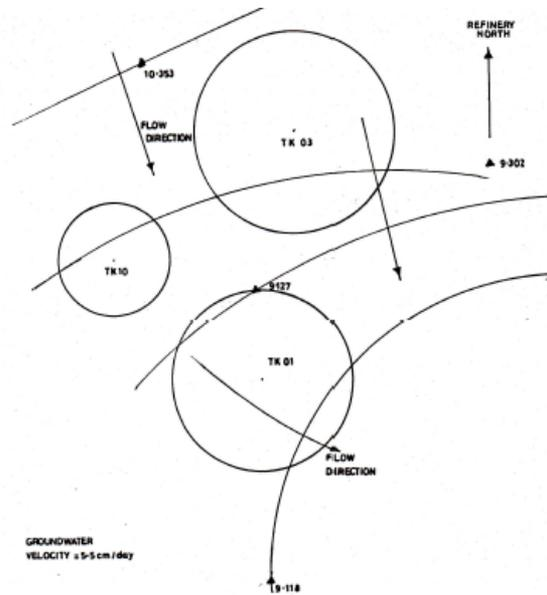
Figure 3: Groundwater flow direction at study site
