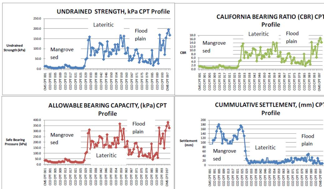
Figure 7: Geotechnical characteristics of some major soils in the Niger delta
