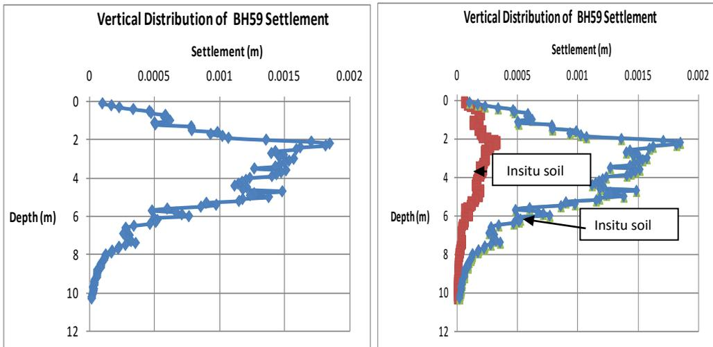
Figure 6: Vertical distribution of settlement before and after soil replacement
