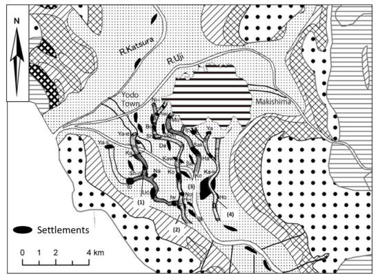
Figure 6: Location of the paleo fluvial channels showing. (1) Sandy gravel fluvial channel.(2) Sandy fluvial channel. (3) Gravel fluvial channel. (4) Paleo Furukawa River fluvial channel. Black distribution is settlements.
