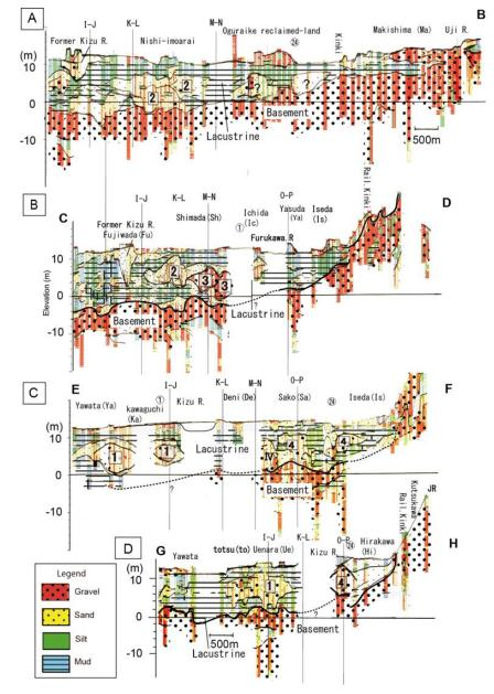
Figure 4: (A)–(D) Geological cross–sections (W–E direction) of the lower reaches of the Kizu River, showing lithology distribution (see location A–B, C–D, E–F and G–H in Figure 1). I–J, K–L and so on show location cross–sections in Figure 5. Boxed numbers are shown in Figure 6.
