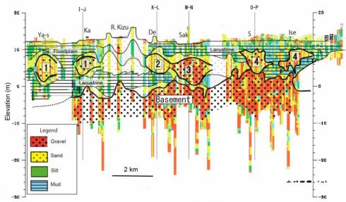
Figure 3: Geological cross-sections (W–E direction) of the lower reaches of the Kizu River, showing lithology distribution (see (1)–(2) in Figure 1 for location). I–J, K–L and so on show location cross-sections in Figure 5. Boxed numbers are shown in Figure 6.
