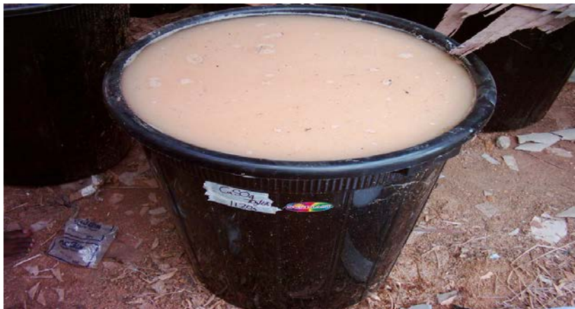
Figure 2: Application of salt solution to soil sample by gravity
