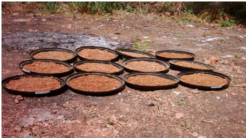
Figure 3: Drying of soil sample prior to permeability test
