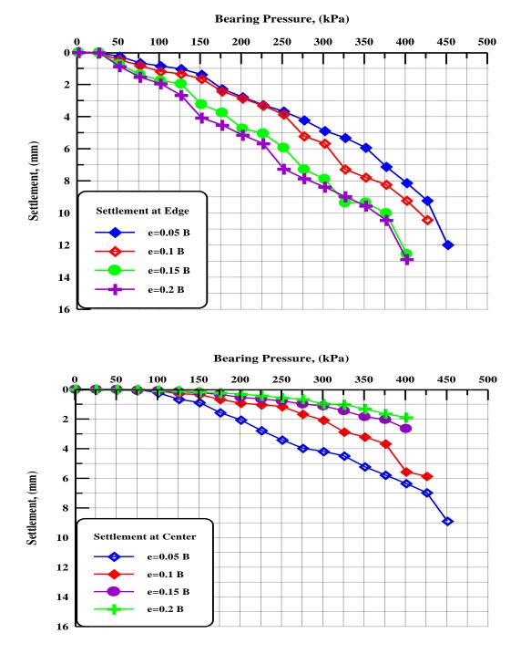
Figure 9: Pressure - Settlement at Edge and Center Curves for Gypseous Soil after Reinforcement on Replaced Soaked Soil. Specific ratio was employed in the tests to investigate the limit of improvement in bearing capacity. This limit represents the ratio between ultimate bearing capacity of gypseous soil replaced by dune sand to the bearing capacity of collapsible soil without replacement. The term was calculated for both reinforced and unreinforced soil.
