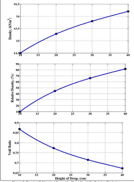
Figure 5: Density Calibration Curves for Dune Sand By Raining Technique.
