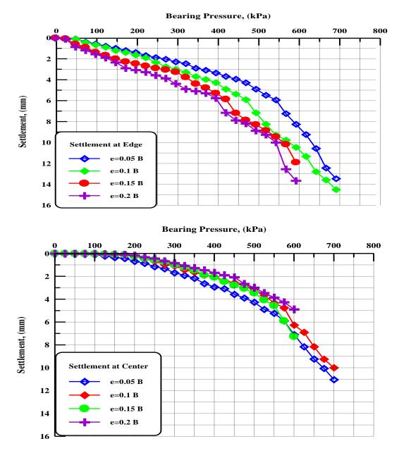
Figure 6: Pressure - Settlement at Edge and Center Curves for Gypseous Soil at Dry State
