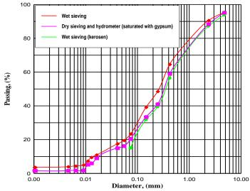
Figure 1: Grain Size Distribution Curves of Gypseous Soil
