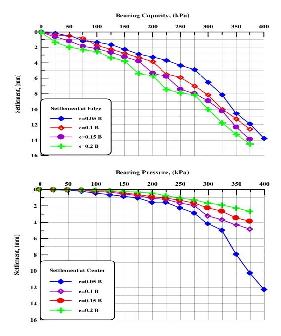
Figure 8: Pressure - Settlement at Edge and Center Curves for Gypseous Soil after Replacement.
