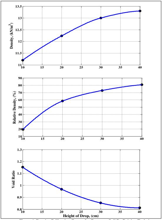
Figure 4: Density Calibration Curves for Gypseous Soil By Raining Technique.
