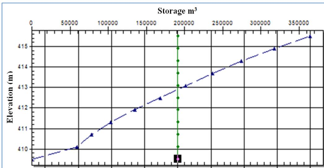
Figure 8-d: Storage-Elevation curve for Reservoir No. 4
