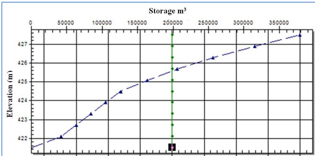
Figure 8-a: Storage-Elevation curve for Reservoir No. 1
