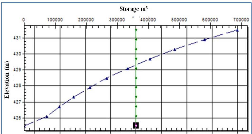
Figure 8-b: Storage-Elevation curve for Reservoir No. 2
