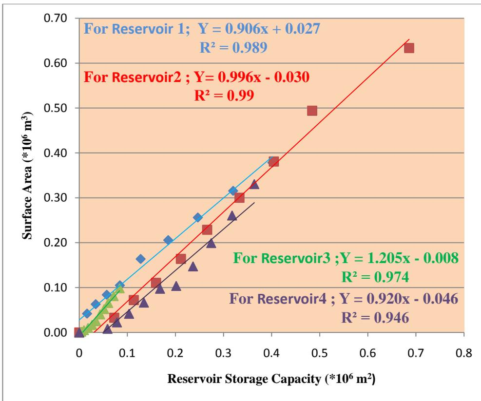
Figure 9: Linearization relationship of Surface area- Storage capacity for the four selected reservoirs.
