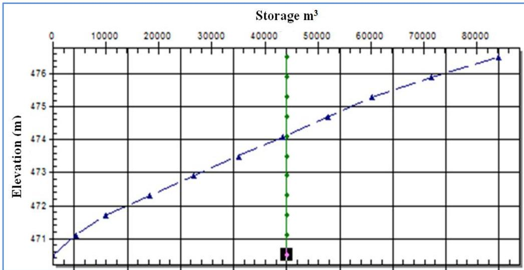
Figure 8-c: Storage-Elevation curve for Reservoir No. 3
