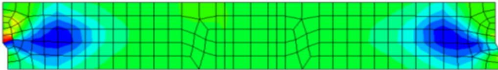
Figure 5: Example of stress distribution in the sheared sample for 1 % shear strain. The scale is in kN/m<sup>2</sup> (kPa).
