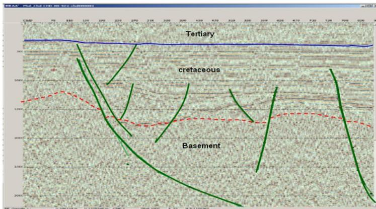
Figure 4: Interpreted seismic profile showing the base Tertiary - top Cretaceous marker and base Cretaceous - Top of the Precambrian Crystalline Basement.
