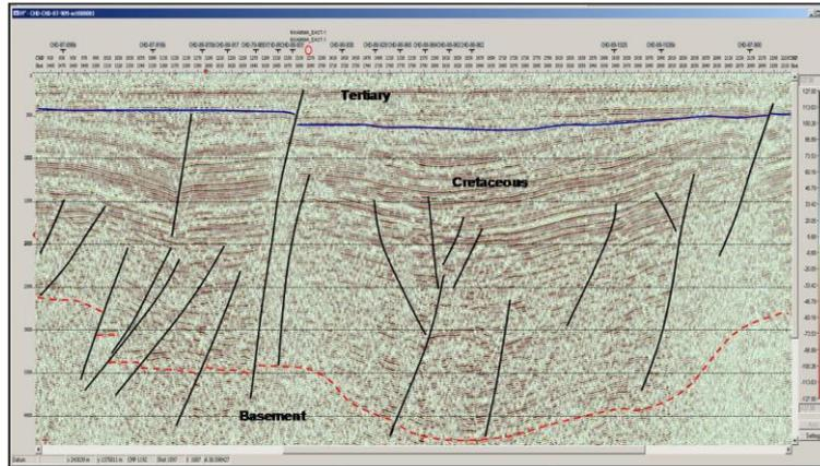
Figure 3: Interpreted seismic profile clearly showing major horizons (Cainozoic, Cretaceous and Basement) and faults
