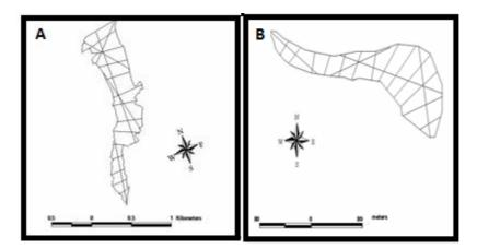
Figure 4: Echo sounding traverses along Burqu(A) and Der Al Kahaf (B) reservoirs.
