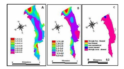
Fig. 8: Sediment at Burqu reservoir. A: mean size (mm), B: sorting (phi), C: skewness
