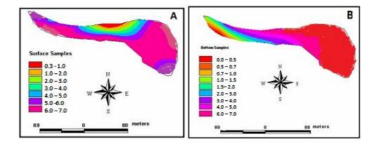
Fig. 12: Suspended sediment concentrations (g/l) at Deir Al-Kahf reservoir, A: surface samples B: bottom samples.
