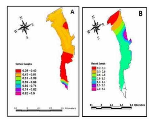
Fig. 9: Suspended sediment concentrations (g/l) at Burqu reservoir, A: surface samples B: bottom samples.
