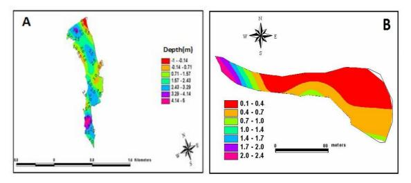
Figure 5: Bathymetric map A: Burqu reservoir B: Deir Al-Kahf reservoir.
