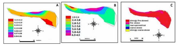
Figure 11: Sediment at Deir Al-Kahf reservoir. A: mean size (mm), B: sorting (phi), C: skewness
