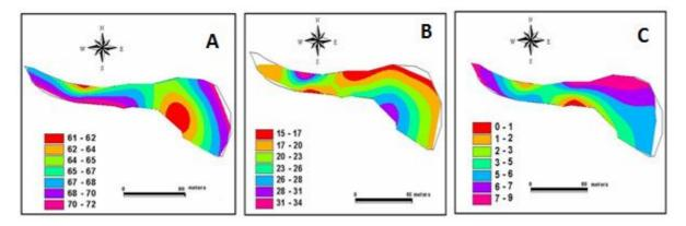
Fig. 10: Sand (A), Silt (B) and Clay (C) percentage distribution at the bed of Deir Al-Kahf reservoir.
