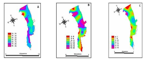
Fig. 7: Sand (A), Silt (B) and Clay (C) percentage distribution at the bed of Burqu reservoir
