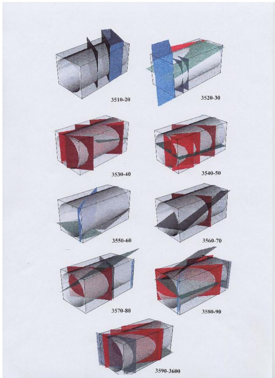
Figure 8. Major water-bearing discontinuities in the Prototype drift illustrating the frequency of intersections of 4<sup>th</sup> order discontinuities, representing “channels”. The interaction of several of these features in the innermost part, i.e. from 3580 to 3600, made up a major fracture zone with strong inflow of water [8].
