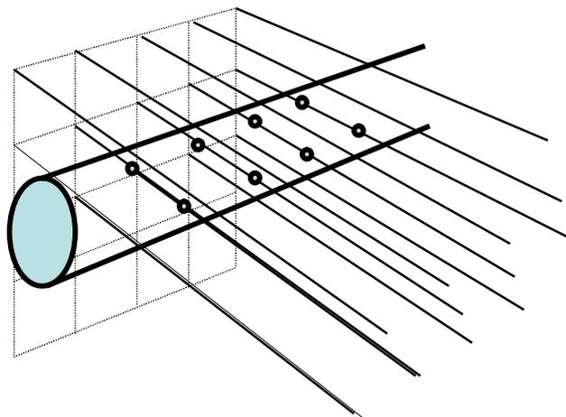
Figure 9. Example of channels formed by intersecting water-bearing fractures grouped in cubical symmetry. The tunnel in the figure happens to fit between two sets of fractures such that only one, sub horizontal, set intersects the tunnel.
