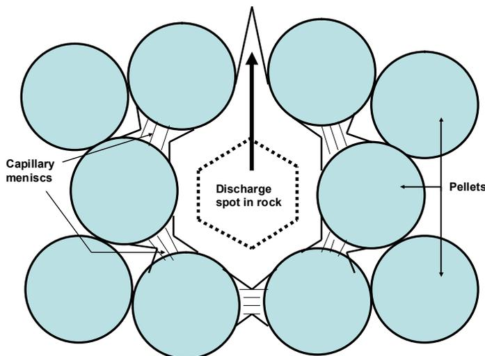
Figure 5. First phase of wetting of the pellet fill at low inflow rate and pressure.
