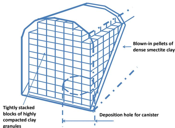
Figure 1. Cross section of tunnel with hole for placement of a HLW canisters according to SKB's concept KBS-3V. The pellet fill has a sloping front.
