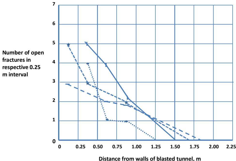
Figure 11. Example of presence of water-bearing fractures in the EDZ of blasted tunnel in granitic rock for different distances from the tunnel contour, determined by mapping of cores taken perpendicularly to the contour [7].
