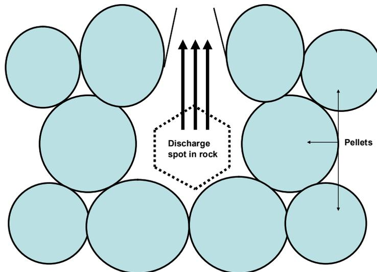
Figure 6. Wetting of the pellet fill at high water pressure.
