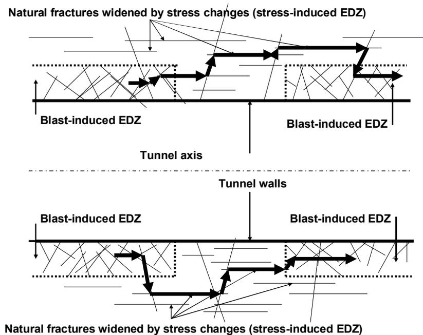
Figure 2. Conceptual model of the creation of an EDZ along a blasted tunnel by hydraulic connection of local blast-induced EDZs and longitudinal natural fractures widened by stress changes. Major flow paths after filling the tunnel with material that is less conductive than the rock are represented by fat arrows.
