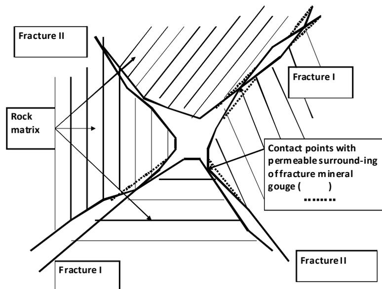
Figure 7. Crossing of fractures (I and II) form a channel that serves as flow path.
