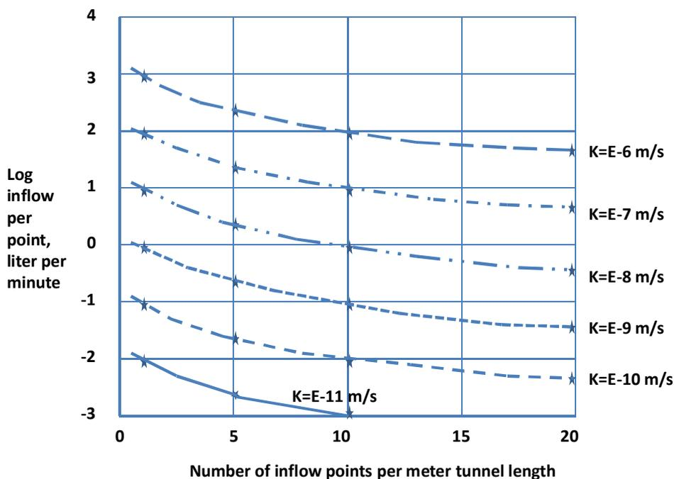
Figure 10. Inflow per point in liters per minute in log scale as function of the bulk hydraulic conductivity of the rock and number of inflow points per meter tunnel length.
