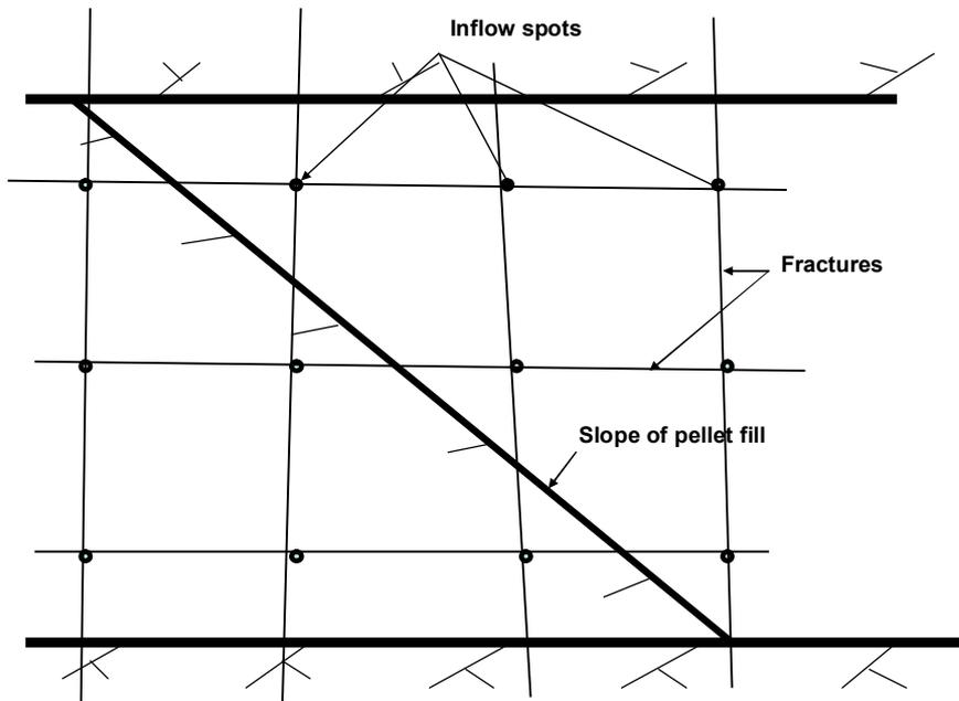
Figure 12. Generalized fracture pattern with inflow points formed by intersecting fractures. The points become located at different distances from the slope in the filling process.
