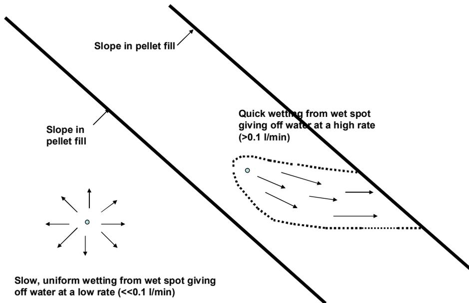
Figure 3. Recorded wetting of smectite pellet fill for different inflow rates from a single inflow point. Left: uniform wetting of the pellet fill for inflow rates  $\ll 0.1$  l/min. Right: Rapid wetting for inflow rates exceeding 0.1 l/min (After Clay Technology AB).
