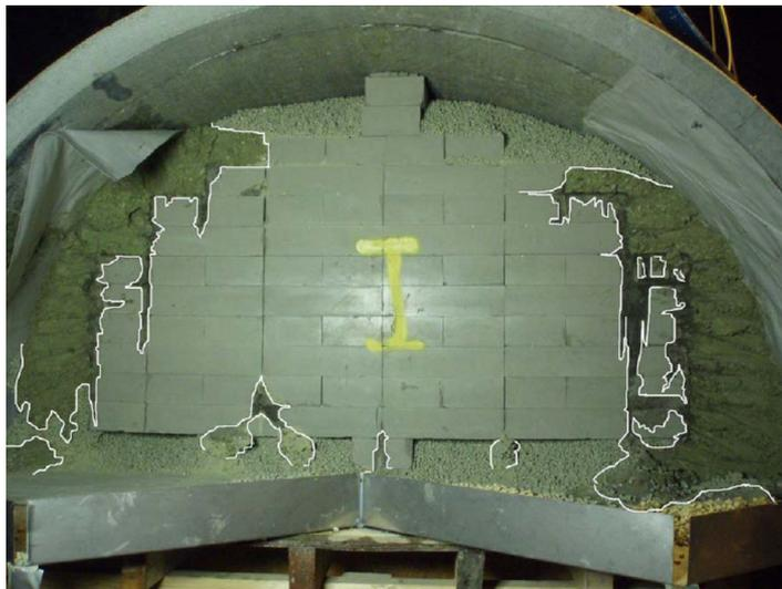
Figure 4. Test for measuring uptake and transport of water in the pellet filling surrounding a clay block assembly. Water was injected at a rate of 0.25 liter per minute in the right part through a nozzle located at the point where the uppermost white line starts, and 0.1 liter per minute in the separated left part through a nozzle hidden by the plastic sheet. In the right part water flowed downwards from start while in the left part it initially tended to flow upwards [11].
