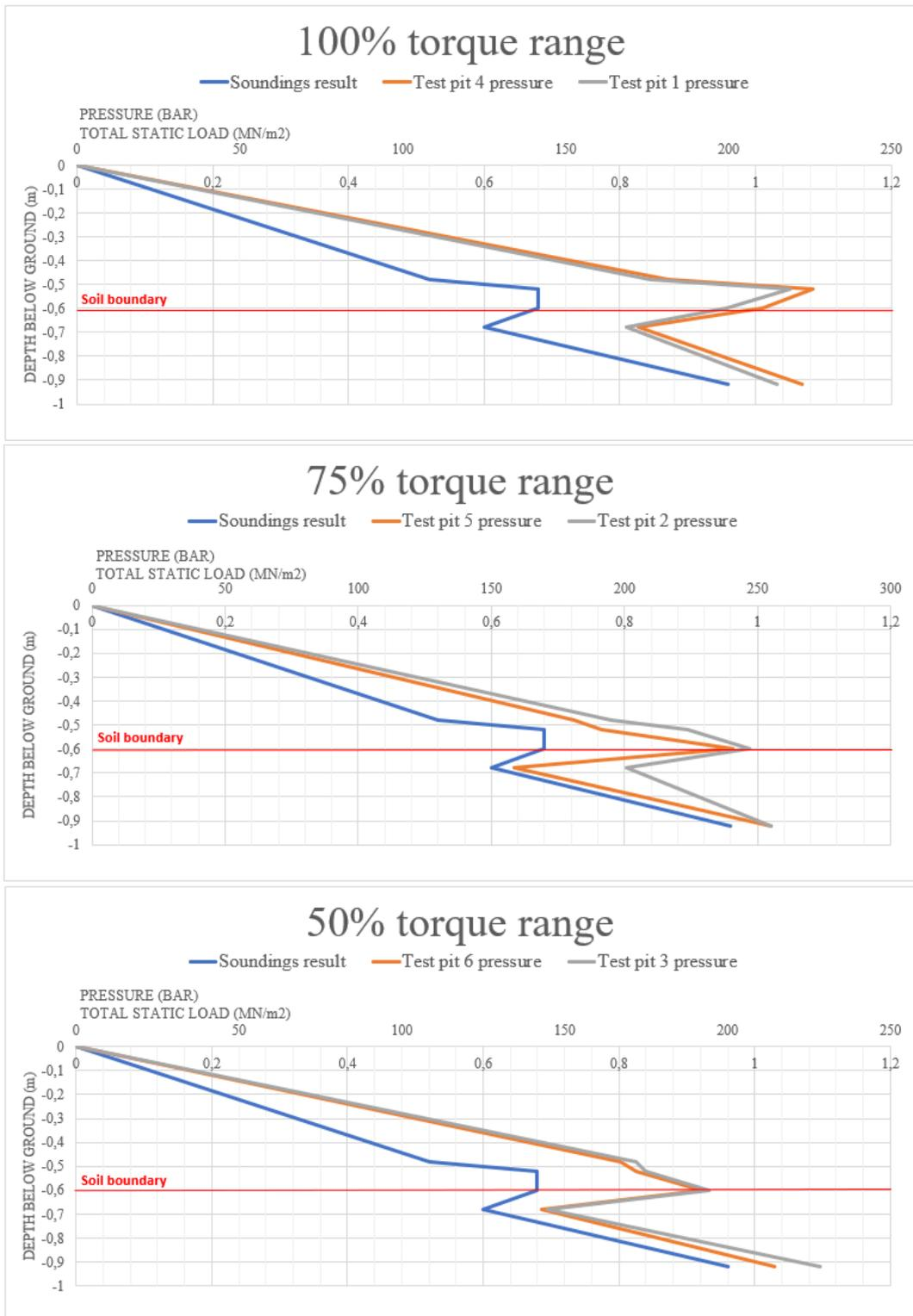
**Figure 4: Correlation results of heterogeneous soil test area per torque limitation range.**
