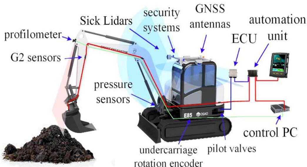
**Figure 1: Layout of the smart excavator used in this study, developed by Oulu University's Civil Engineering Research Unit (Immonen et al., 2021).**
