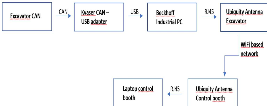
**Figure 3: Signal output sequence of excavator engine data.**
