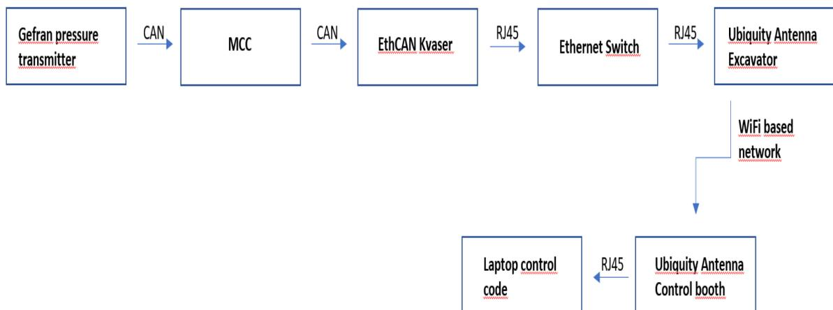
**Figure 2: Signal output sequence of Gefran pressure transmitters.**
