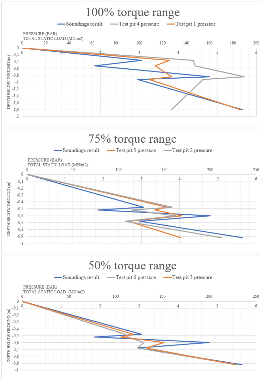
**Figure 5: Correlation results of homogeneous soil test area per torque limitation range.**
