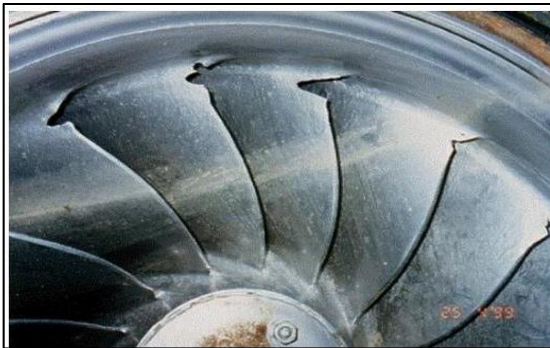
Figure 15: Sedimentation abrasion of the turbine runners at the Jhimruk hydropower plant, Nepal [22].
