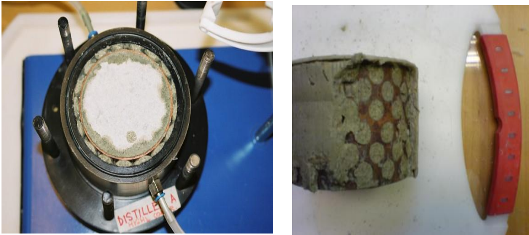
Figure 6: Maturation 4 of clay seal. Left: Clay expanded radially through the perforated tube by adsorbing low-electrolyte water for 8 hours. Right: 24 hour old seal of dense clay in smectite clay mud with an initial dry density of 200kg/m 3 .
