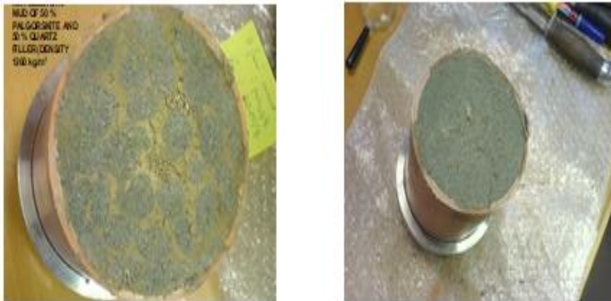
Figure 10: Borehole seal of smectite granules mixed into mud. Left: Sectioned sample at start of water uptake. Right: Largely homogeneous state after 40 days (Pusch et al, 2011).
