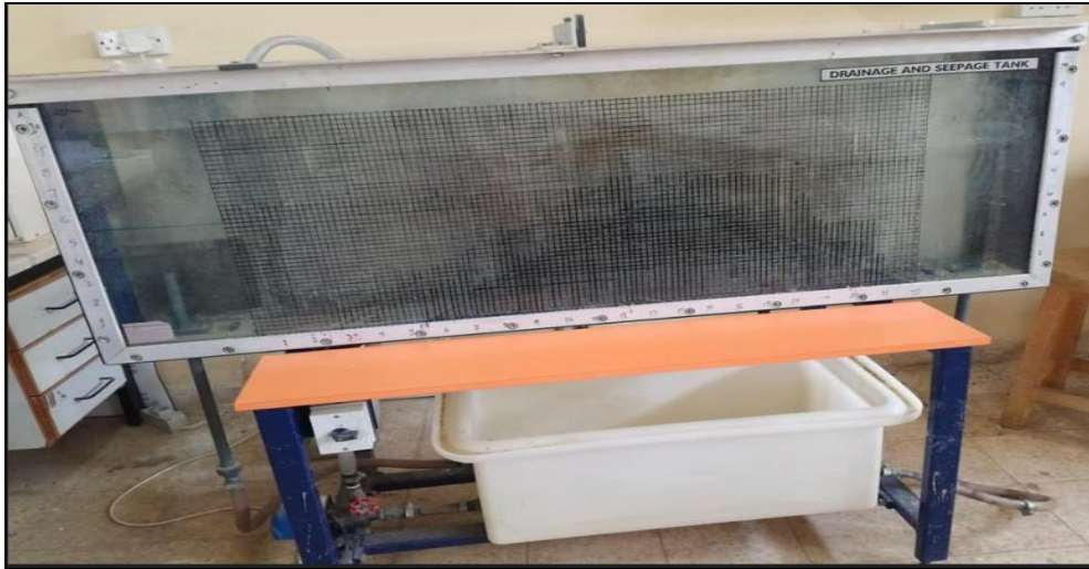
Figure 1: The Seepage and Drainage Apparatus
